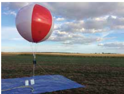
Automated bat detector attached to a balloon for bat activity survey during EIA. © J. Sudraud
